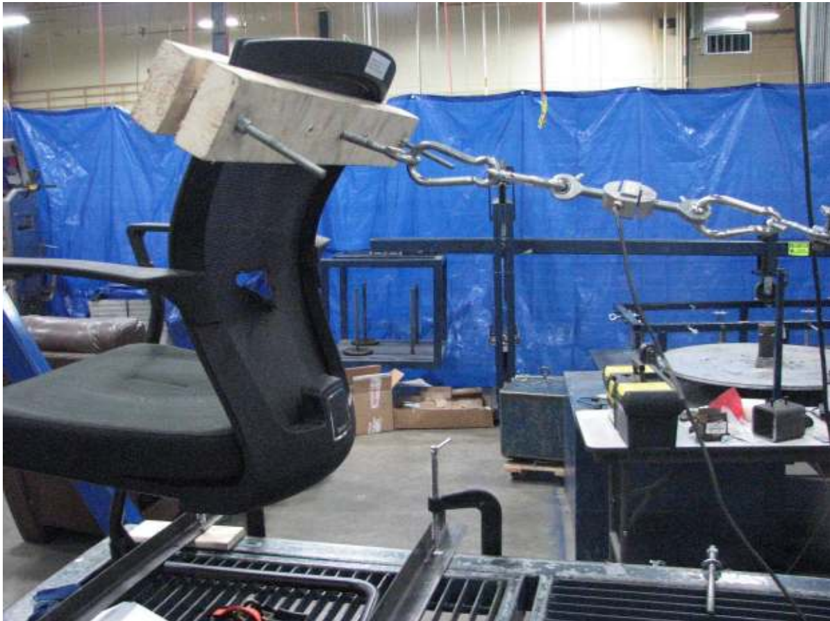
BACK STRENGTH PROCEDURE - STATIC
