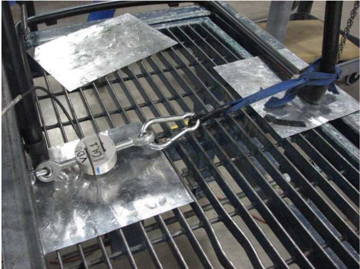
LEG STRENGTH TEST - SIDE APPLICATION
