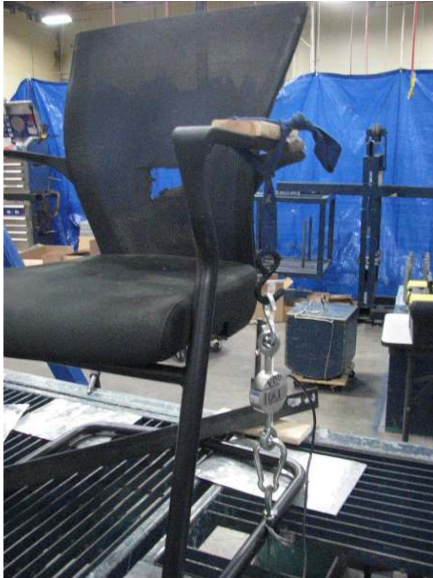
Arm Strength Test Vertical-Static
