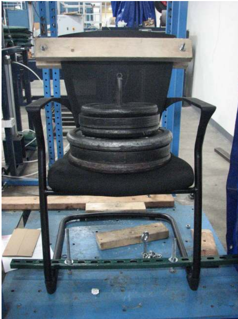
BACK DURABILITY TEST-CYCLIC
