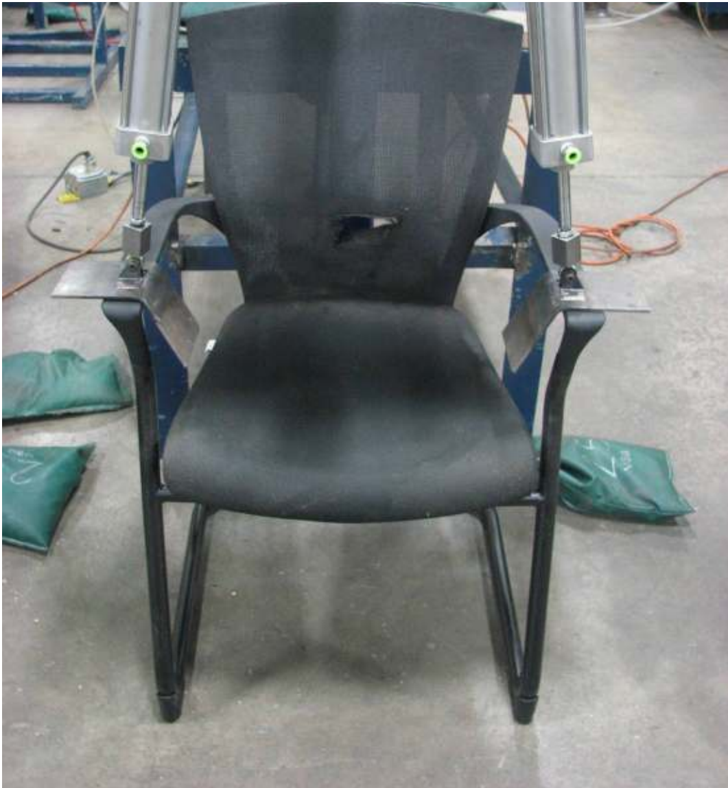
Arm Durability Test – Cyclic
