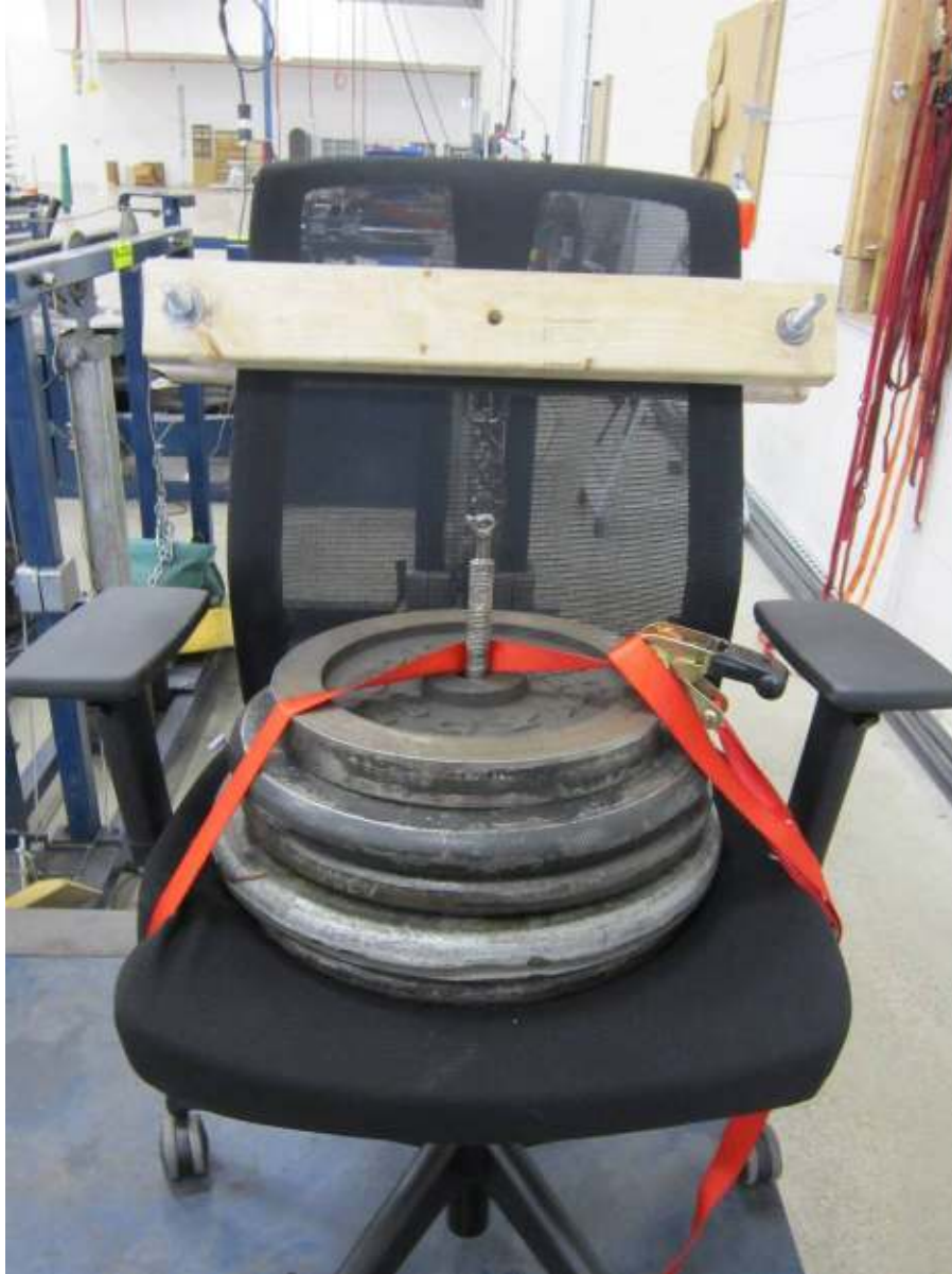
Tilt Mechanism Test-Cyclic
