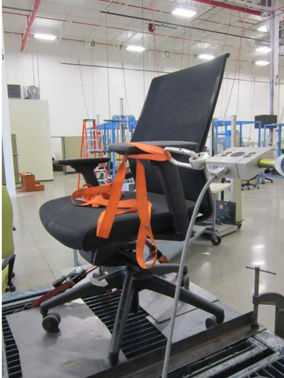
Arm Strength Test- Horizontal-Static
