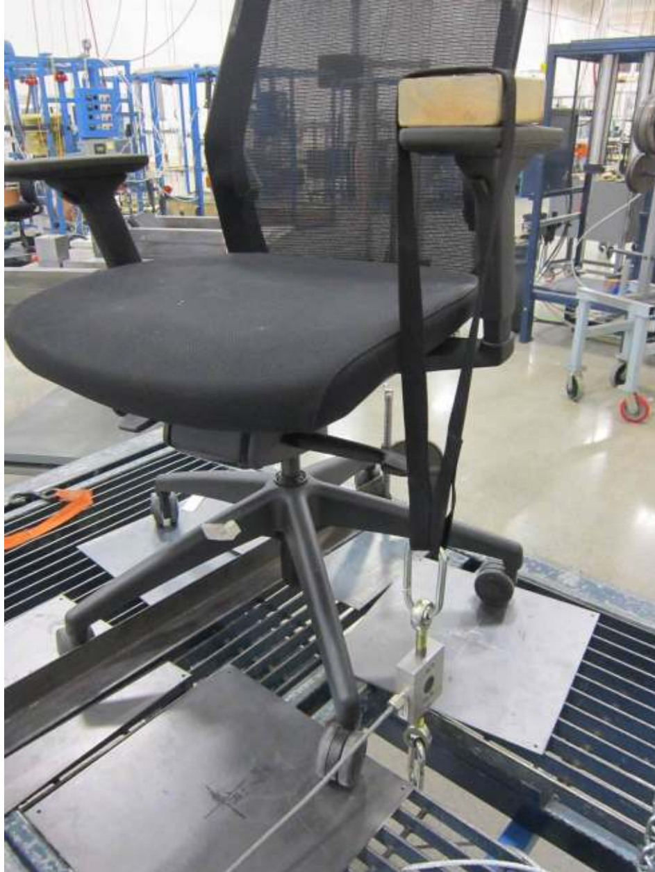
Arm Strength Test Vertical-Static
