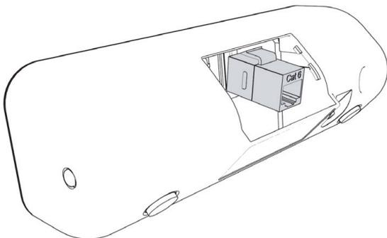
Insert the data connector so that the ridge on its lower face engages with the step on the aperture...
