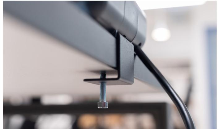
Attach the bracket to the back of the UNO module and place on a table edge. Then tighten to secure the UNO by using a 5mm allen key. The standard bracket size is 25 - 30mm, a larger 50mm bracket is available upon request. A packer bracket is also available to lift up the UNO for larger chargers.
