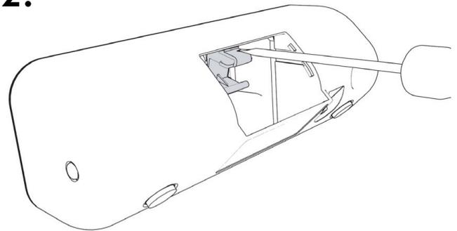
Carefully unclip the data blanking-plate using a flat-bladed screwdriver and store in a safe place.
