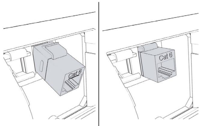
...then push firmly forwards to engage the flexible clip.
