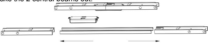
Put the legs into the assembly frame for the controller, and ensure that the side with screw holes for assembly frame beam are put upwards. Align the holes on the legs and holes on the assembly frame, fasten 4 M6\*10 hex screws with M4 Allen wrench. If screws are accidentally dropped into the assembly frame, incline the frame, and the screws could be take out easily.
