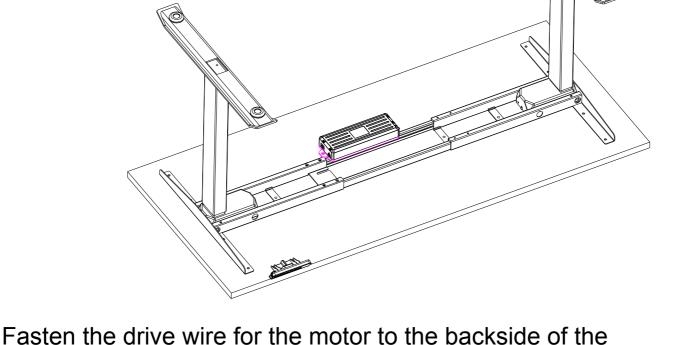
desktop with clamps with gum, and tighten the clamp to prevent it from falling. The wire could be organized based on the personal needs, and fasten the cap to the central beam with 8 M6\*10 hex screw.
