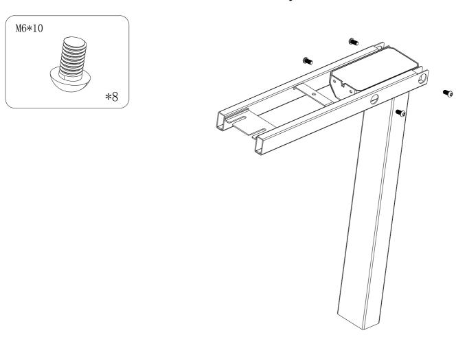
Put the side bracket into the assembly frame for the controller, and fix them with 2 M6\*14 hex screws.
